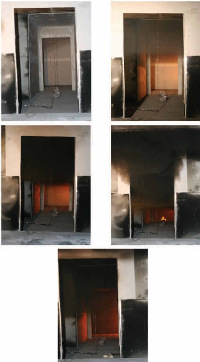
Figure A-6. Example Fire Progression from Test CRA 1
